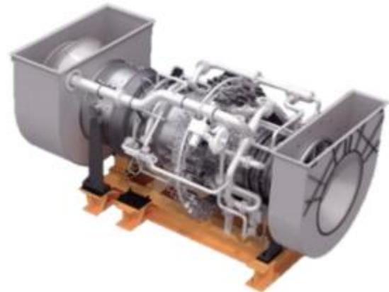
Engine inspection and overhaul is performed in a workshop. The engine module has been designed to be easily and quickly removed from the package. All the engine electrical connections are wired to two Junction Boxes installed on the engine support structure.
