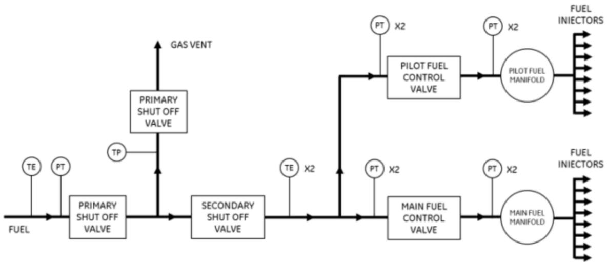
*Typical fuel system schematic*
