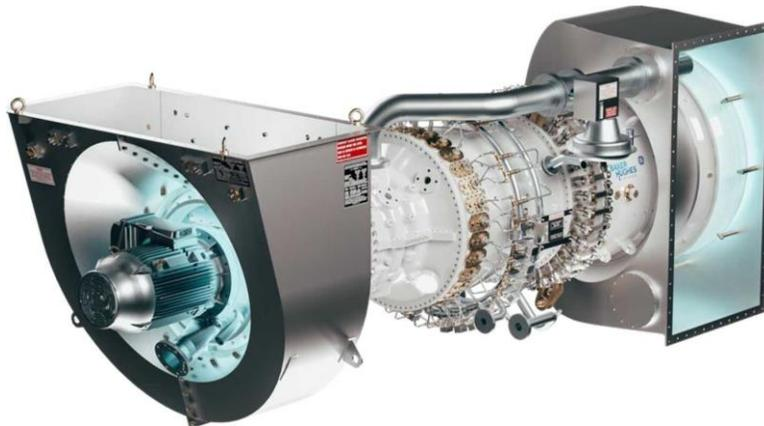
Air entering the inlet section of the gas generator is directed into the axial compressor by the inlet casing, and then compressed to a ratio of 19:1 (nominal rating at ISO conditions).
