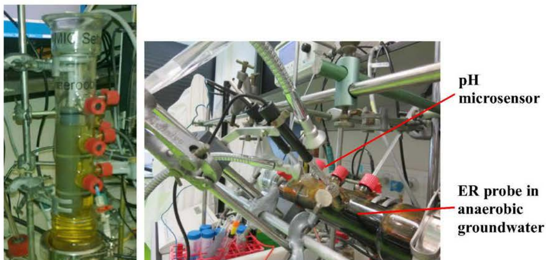
Figure 2: Left: ER probe in anaerobic reactor containing groundwater; right: close-up of setup for measurement for gradients using microsenors.
