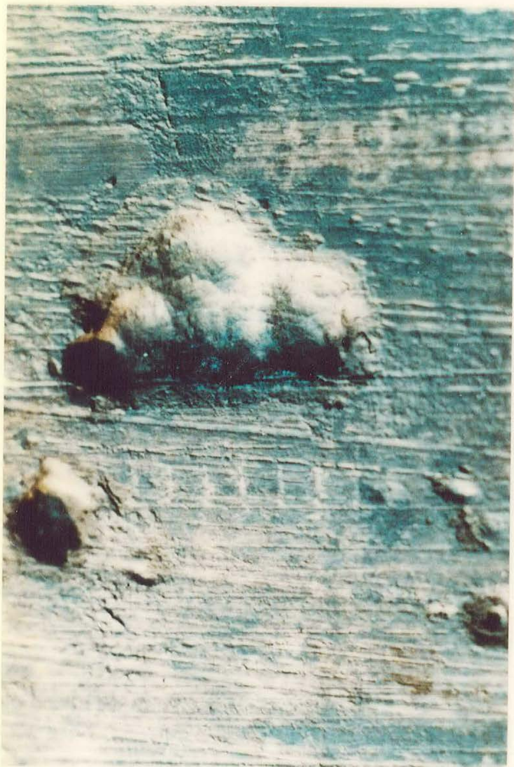
Figure 13 Same Pit After Cleaning with Nylon Brush (Note Cup-like Pits Inside Large Pit)
