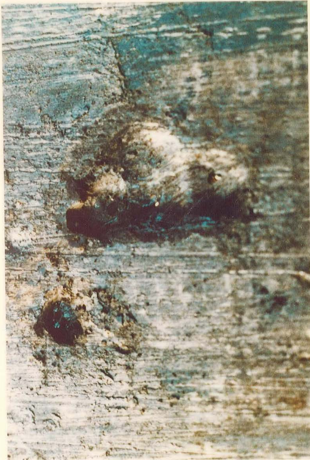
Figure 12. Same Pit After Corrosion Product is Scraped Out
