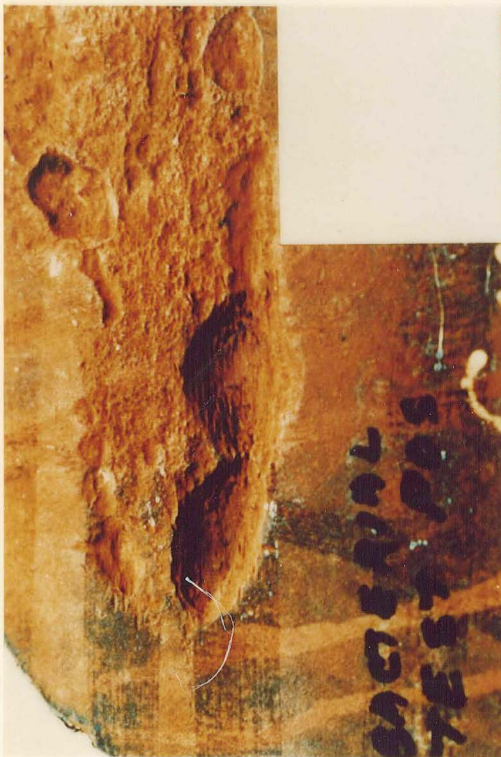
Figure 9. Corrosion Pits with Striations
