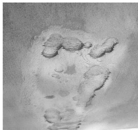
Fig. 10 Microbially induced corrosion showing striations in the bottom and tunneling into the walls of overlapping pits, as described in Ref 32
