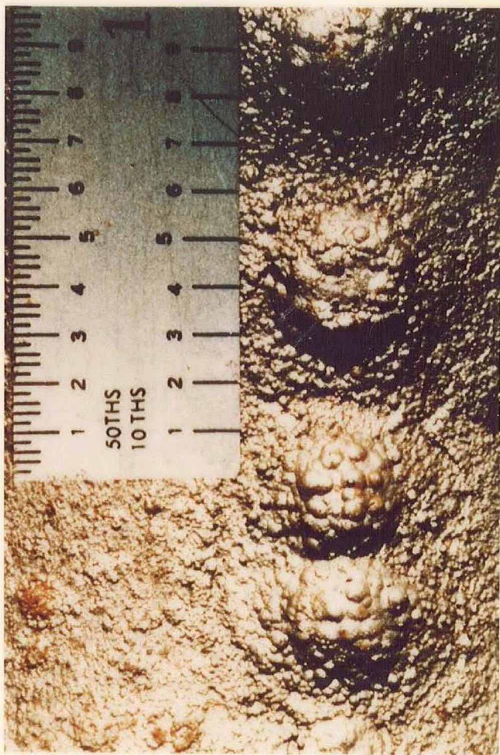
Figure 8. Cup-type Scooped Out Hemispherical Pits on Flat Surfaces with Craters in Pits
