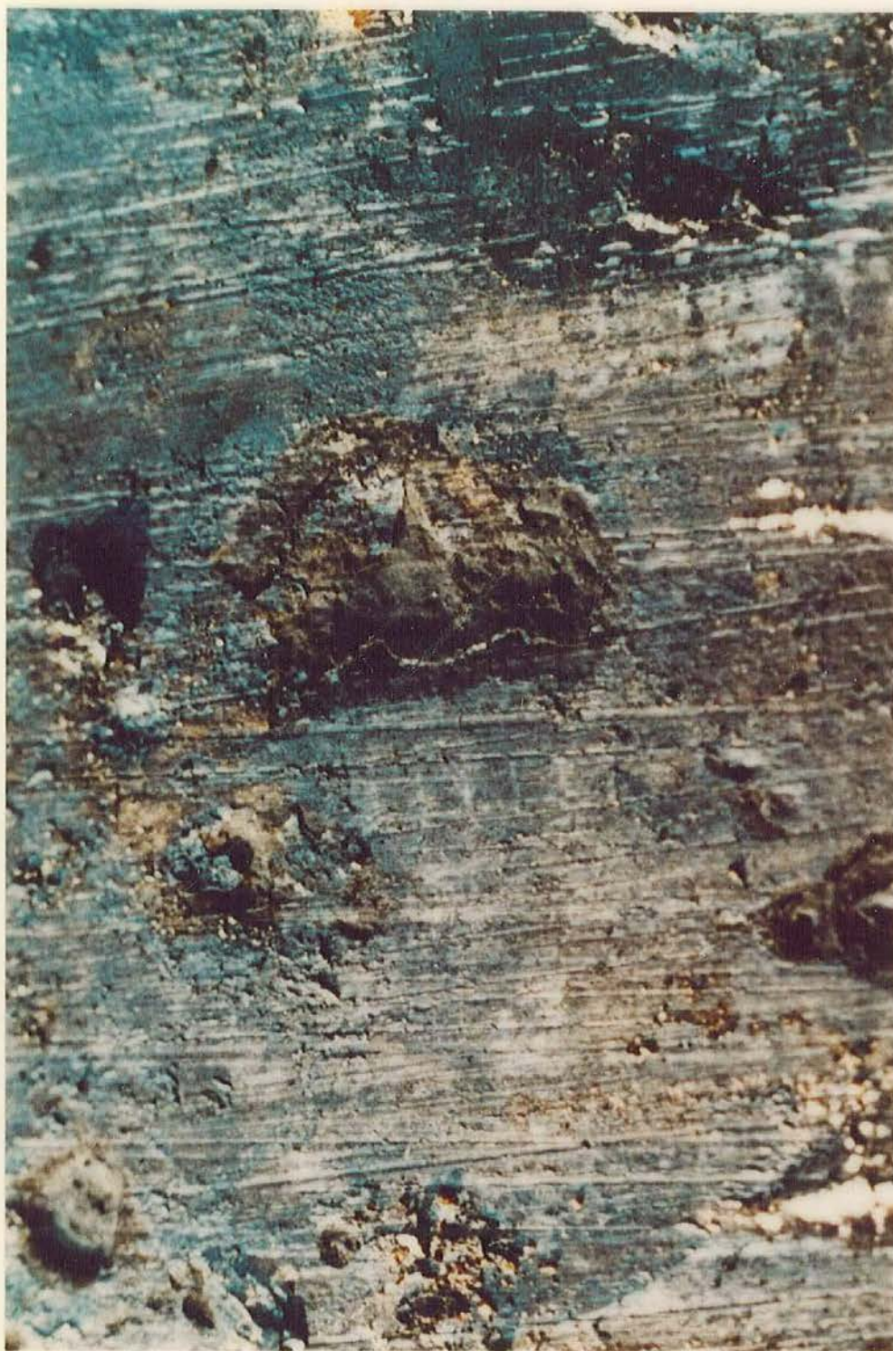
Figure 11. Surface Pit Showing Corrosion Product in Pit
