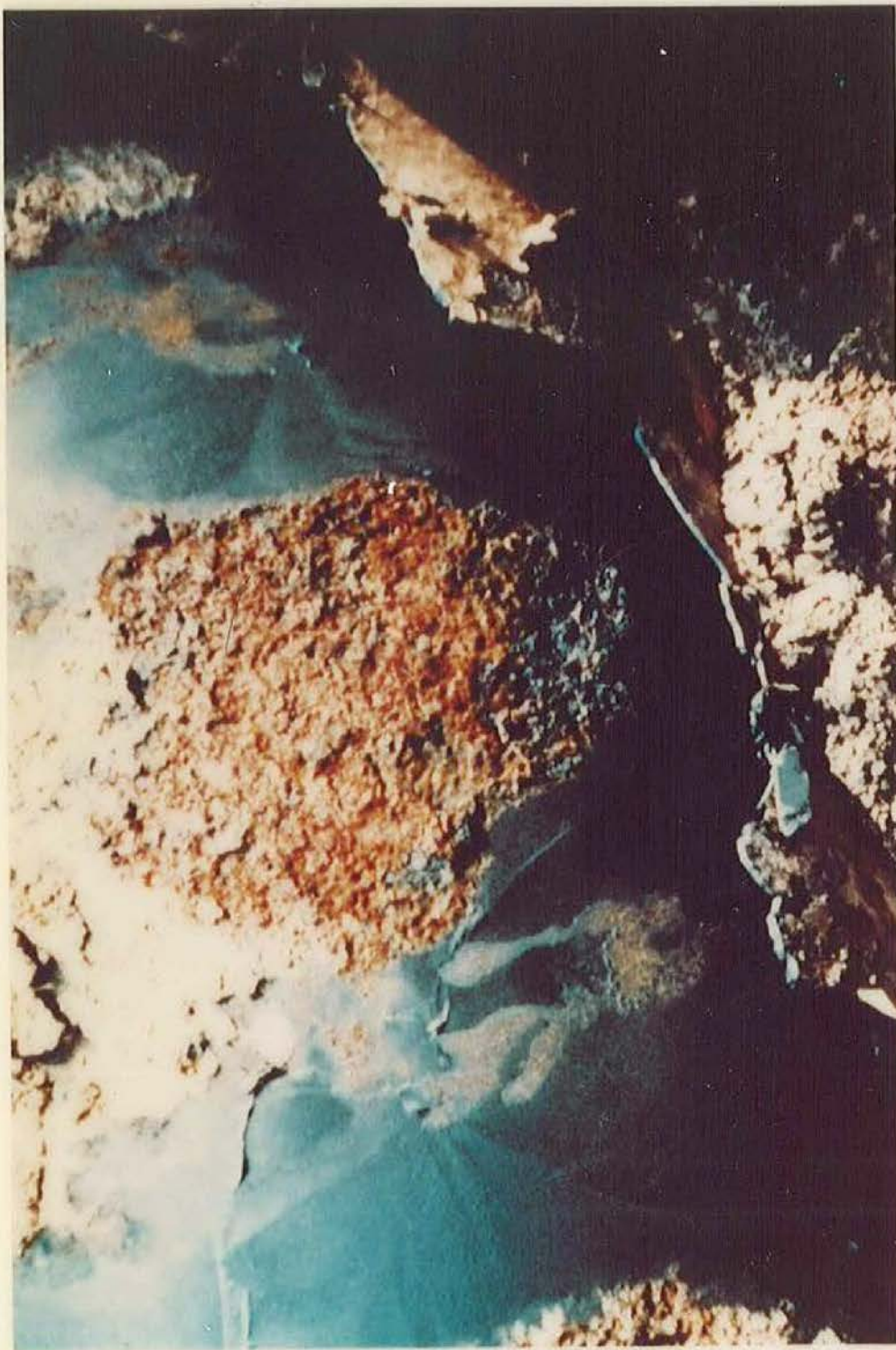
Figure 1. Localized External Corrosion with Deposits, Pits, Craters and Some General Attack
