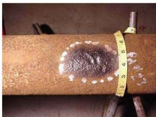
Figure 12 - Digital image showing the defect where Example 3 physical measurements were taken.
