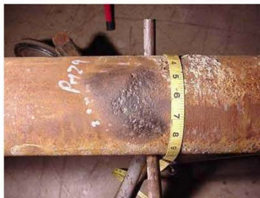
Figure 15 - Digital image showing the defect where Example 4 physical measurements were taken.
