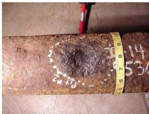
Figure 6 - Digital image showing the defect where Example 1 physical measurements were taken.
