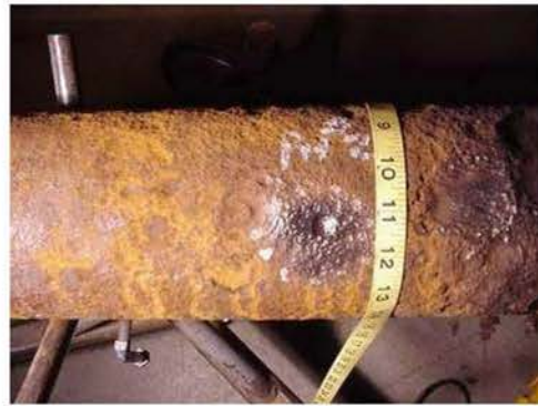
Figure 18 - Digital image showing the defect where Example 5 physical measurements were taken.
