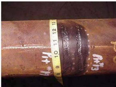
Figure 29 - Digital image showing the defect where Example 9 physical measurements were taken.
