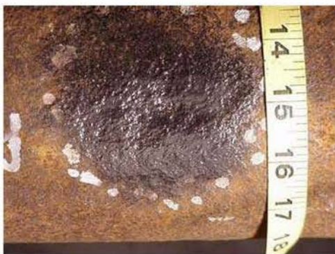
Figure 20 - Digital image showing the defect where Example 6 physical measurements were taken.
