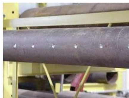
Figure 2 - Manufactured defects used for calibration.
