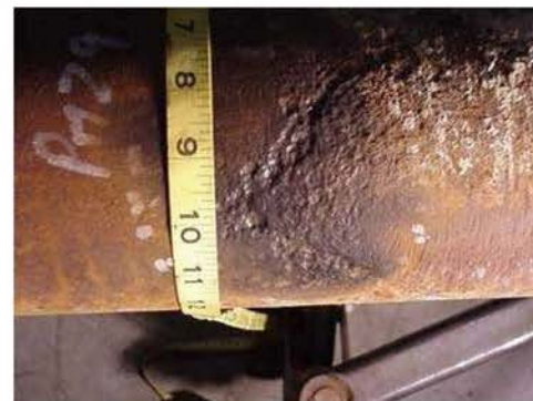
Figure 14 - Digital image showing the defect where Example 4 physical measurements were taken.
