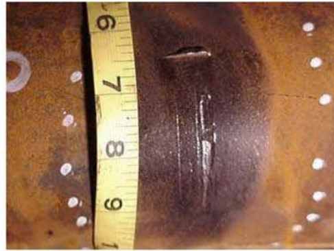
Figure 27 - Digital image showing the defect where Example 8 physical measurements were taken.
