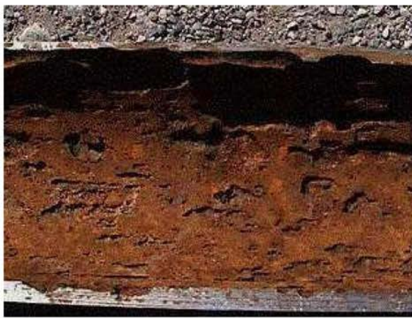
Fig. 18: WELL-0057 Tubing joint box end corroded section
