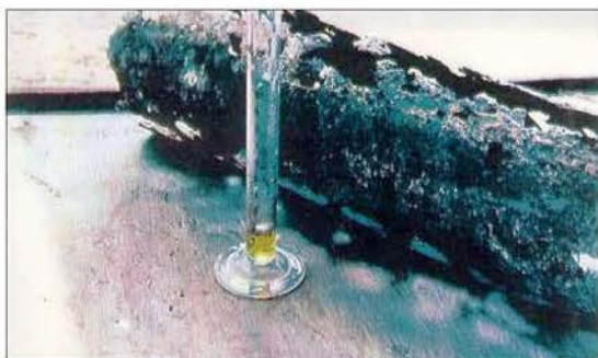
Fig. 15: Piece of WELL-0043 pulled out tubing showing severe damage
