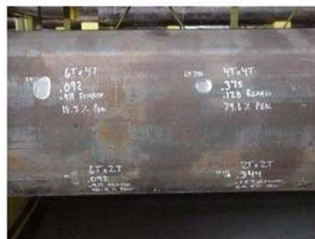
Figure 1 – Manufactured defects used for calibration.
