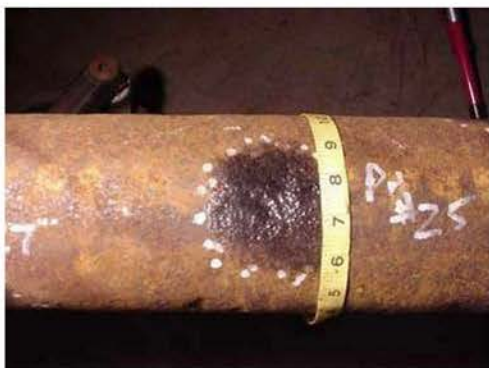
Figure 21 - Digital image showing the defect where Example 6 physical measurements were taken.
