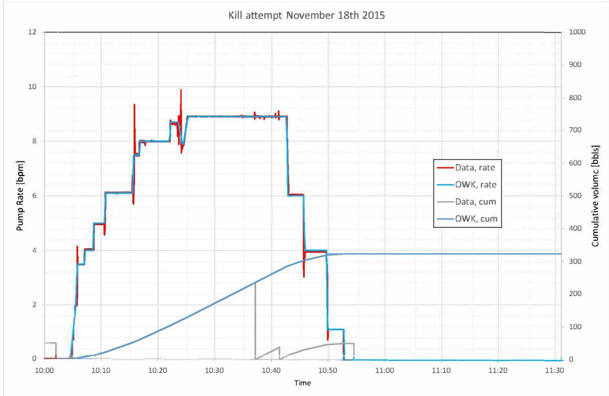
Figure 6.9: Pump rates during pumping operation November 18<sup>th</sup> 2015
