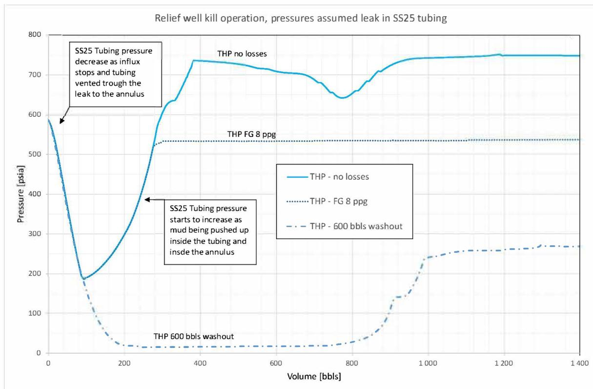
Figure 7.14: Example of relief well kill scenarios assuming hole in tubing
