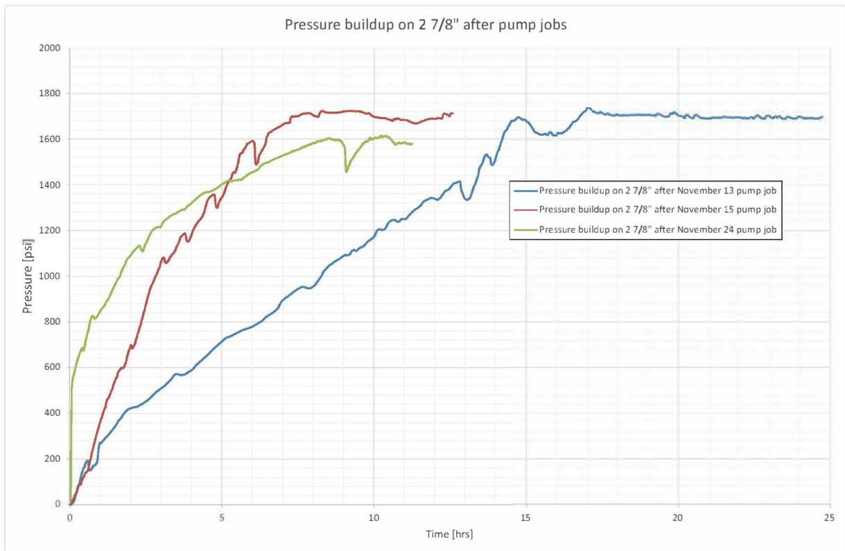
Figure 6.16: Pressure build-up on tubing after kill jobs
