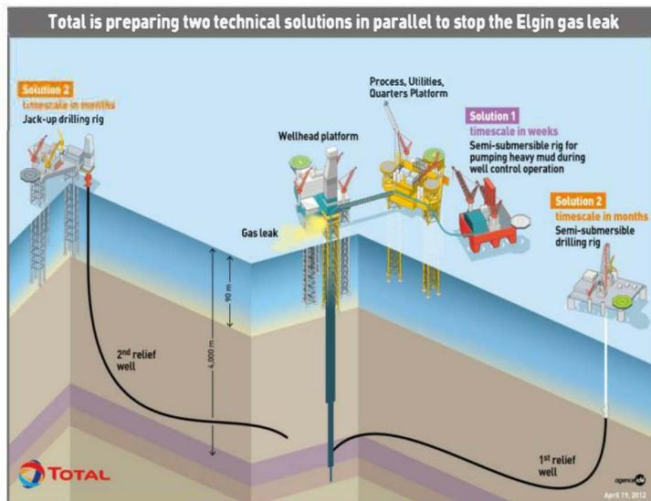
The blowout occurred during P&A of a HPHT production well on the Elgin wellhead platform in the UK sector of the North Sea. The well flowed gas and condensate to the platform deck due to mechanical failure of all casing strings after pressure build-up. A successful surface intervention followed by dynamic kill was possible due to low flow rate of gas and condensate. All personnel safely evacuated.
