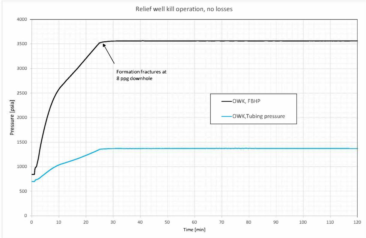
Figure B.10: Pressure response curves, RW kill, fracture gradient of 8 ppg
