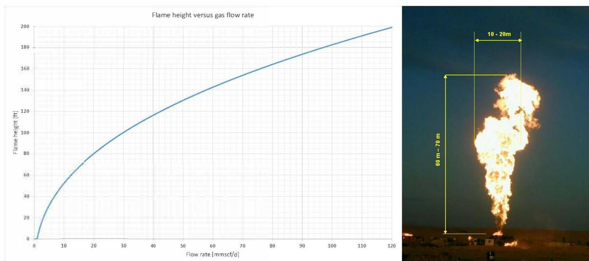
Figure 3.7: Flame height versus flow rate, and gas blowout in Algeria in 2000
