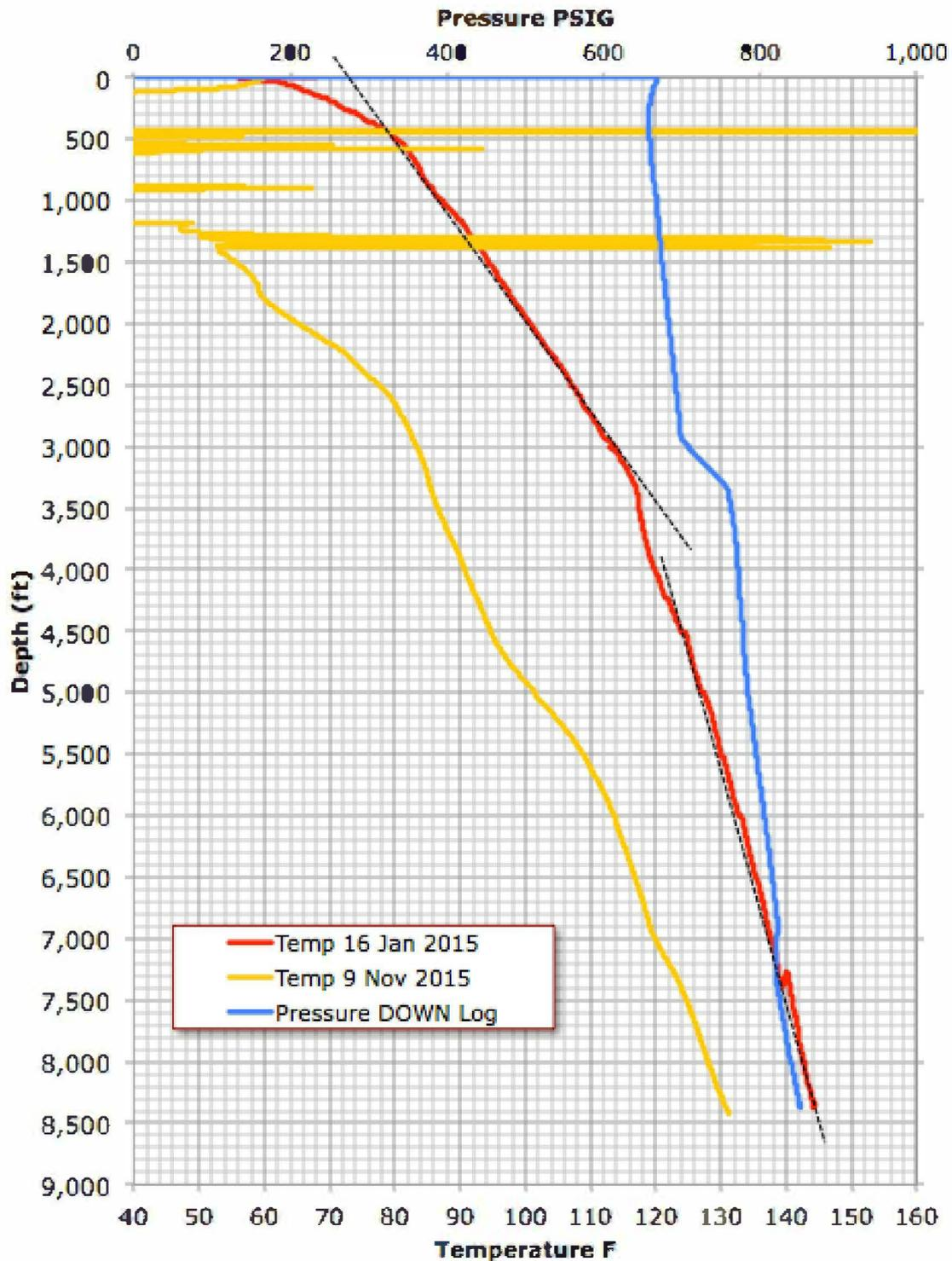
Figure 2.7: Pressure and temperature log from November 9 and January 16<sup>th</sup> 2016
