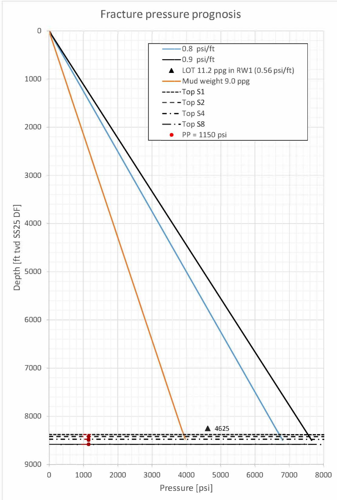
Figure 1.5: Fracture pressure prognosis
