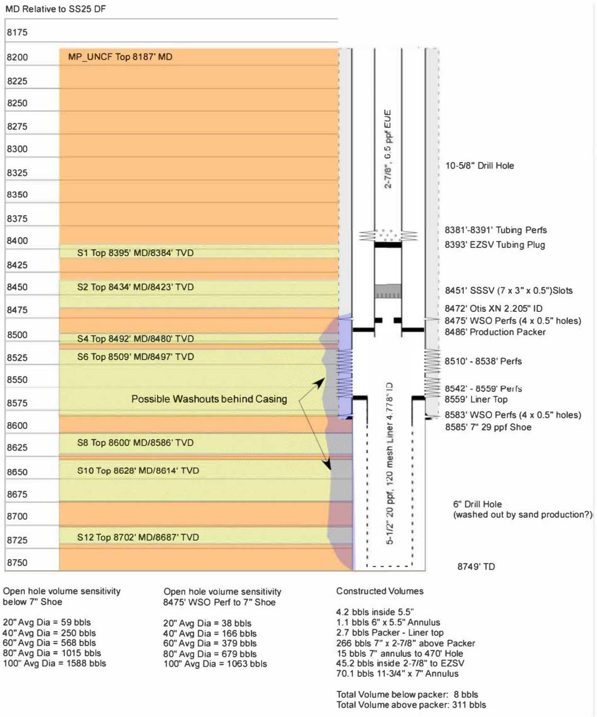
Figure 1.9: Details of the lower completion and reservoir sands
