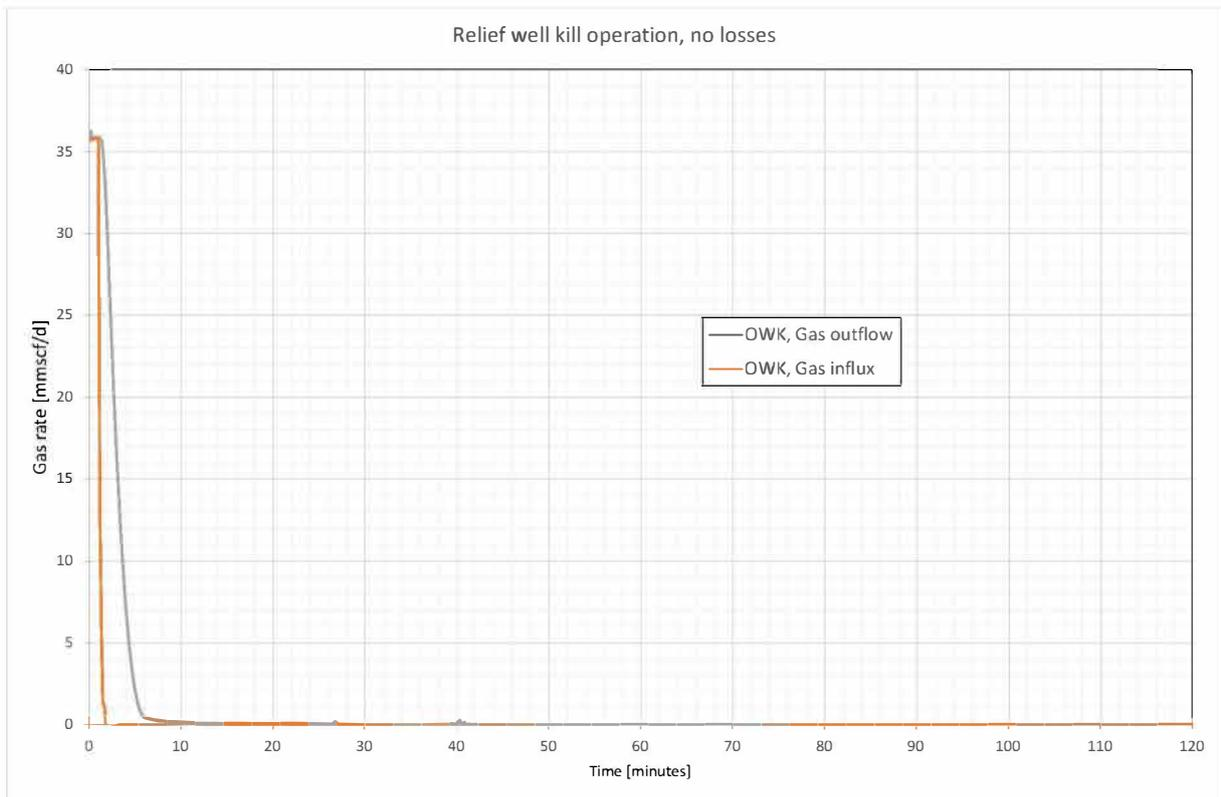
Figure B.11: Flow rates, RW kill, no losses, fracture gradient of 8 ppg
