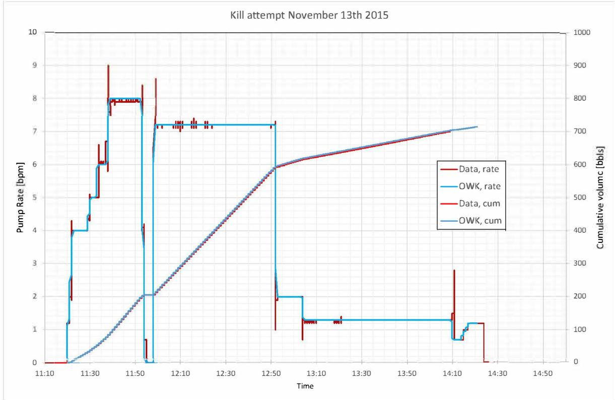
Figure 6.2: Pump rates during pumping operation November 13<sup>th</sup> 2015
