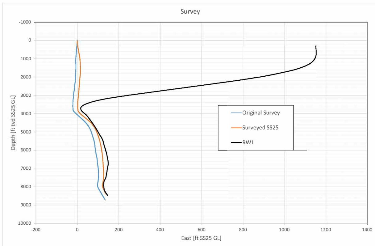
Figure 7.4: Relief well trajectory, East – TVD
