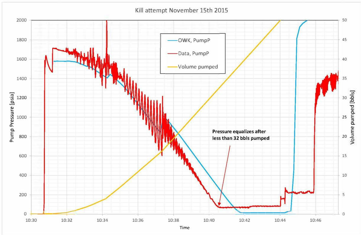
Figure 6.8: Pressure step-down during pumping operation November 15<sup>th</sup> 2015
