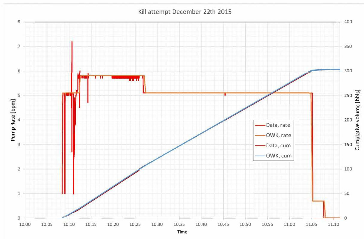
Figure 6.18: Pump rates during pumping operation December 22<sup>nd</sup> 2015
