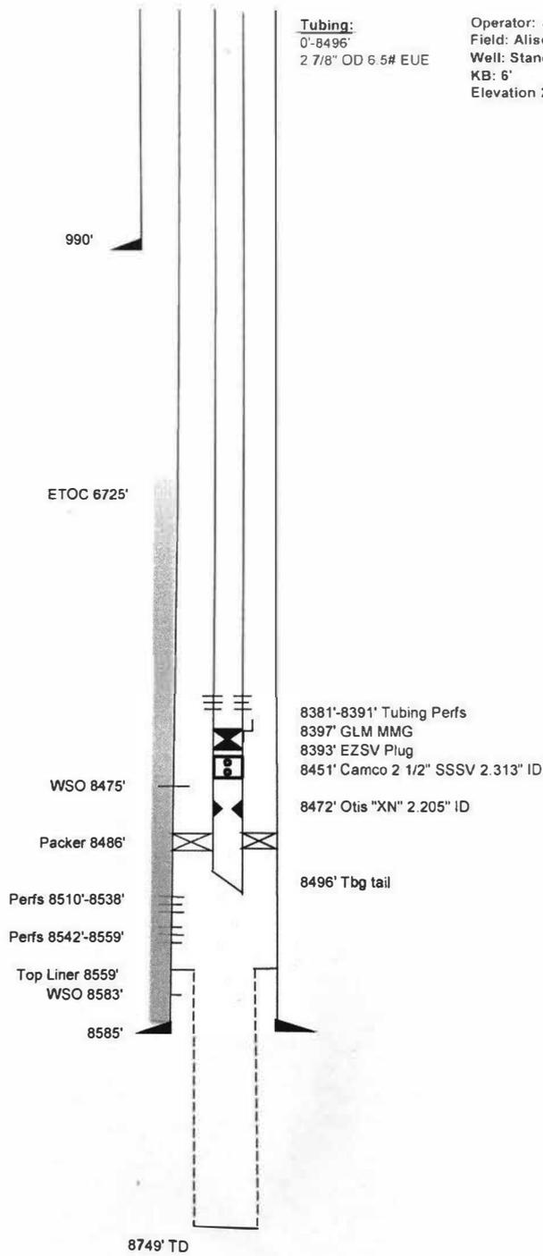
Figure 1.8: Wellbore schematic after tubing being perforated
