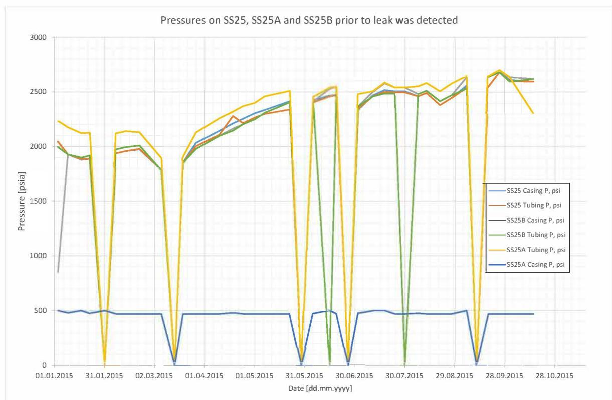
Figure 2.1: Recorded pressures on SS25, SS25A and SS25B prior to leak
