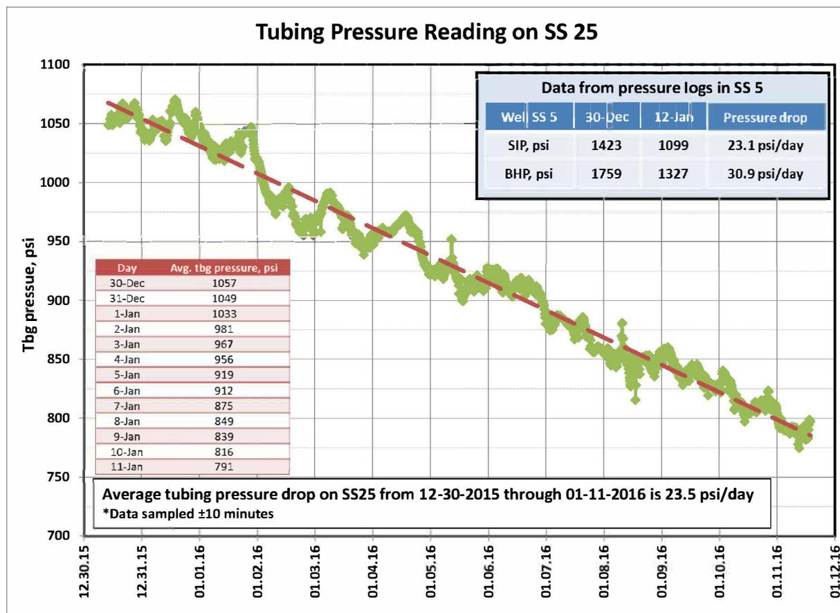
Figure 2.4: Tubing pressure reading on SS25
