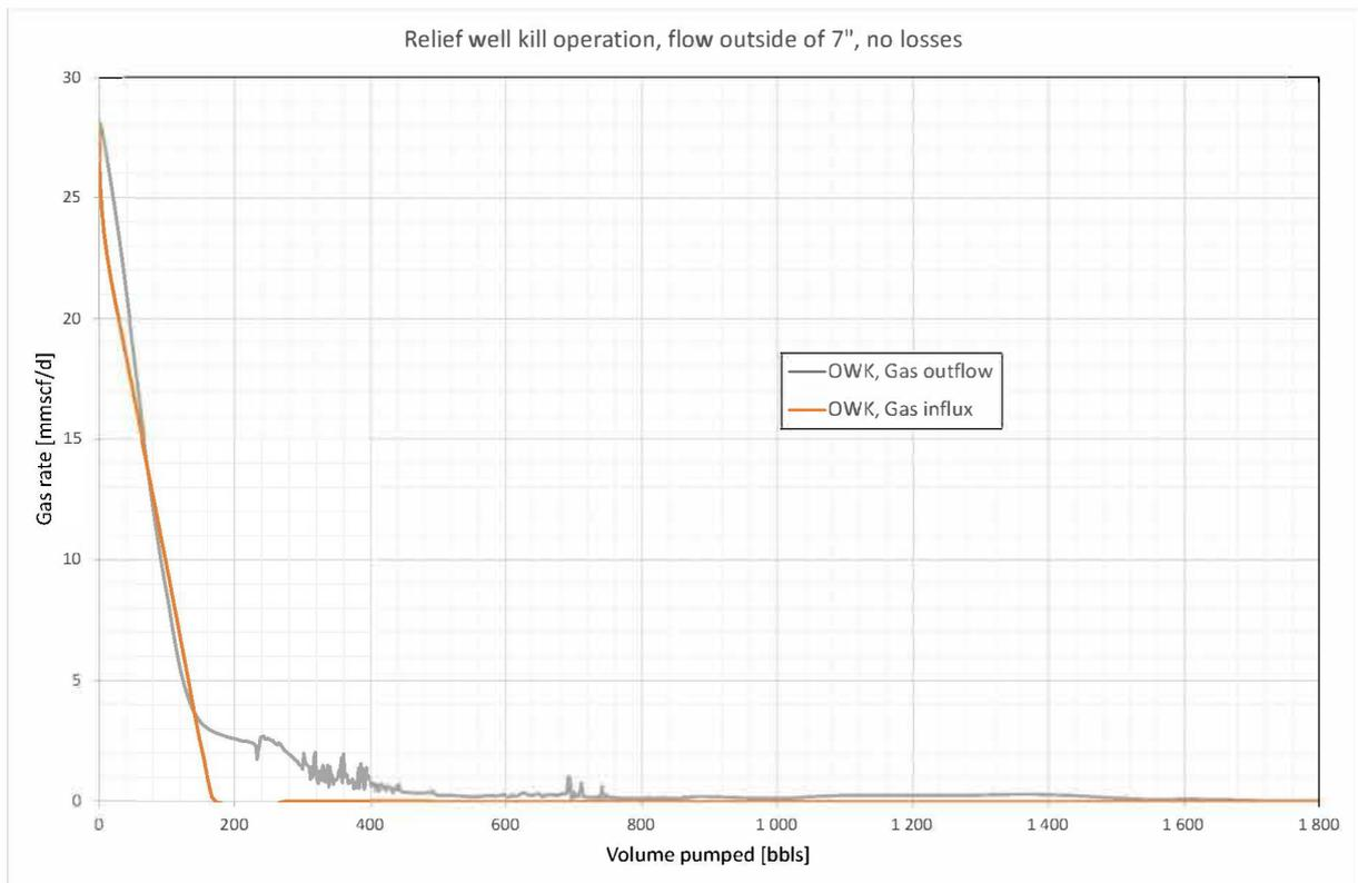
Figure 7.16: Gas rates during RW kill assuming flow outside the 7" csg
