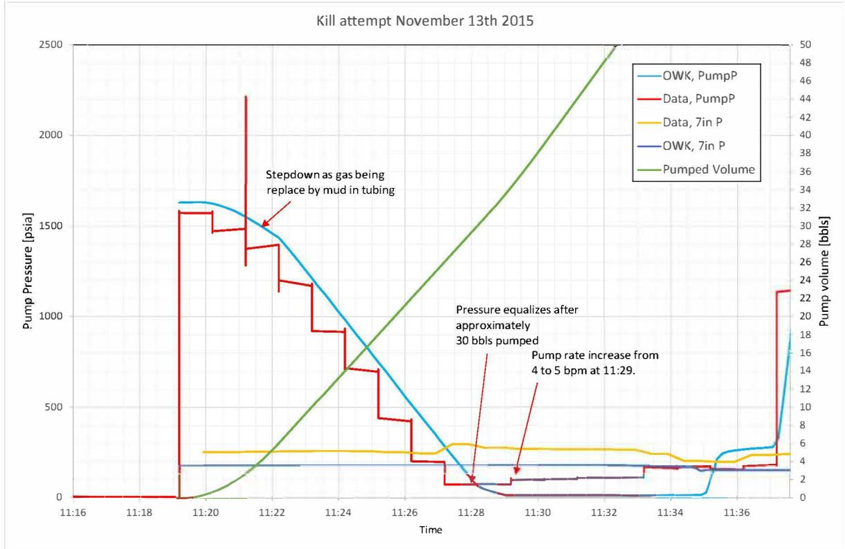
Figure 6.4: Pressures step-down during operation November 13<sup>th</sup> 2015
