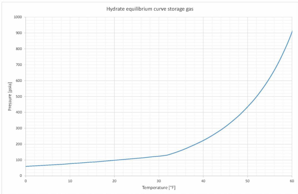
Figure 3.6: Hydrate equilibrium curve for storage gas
