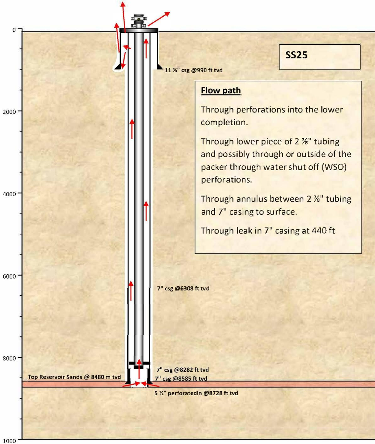
Figure 3.3: Schematic of potential flow path in annulus between 7" csg and 2 7/8" tbg
