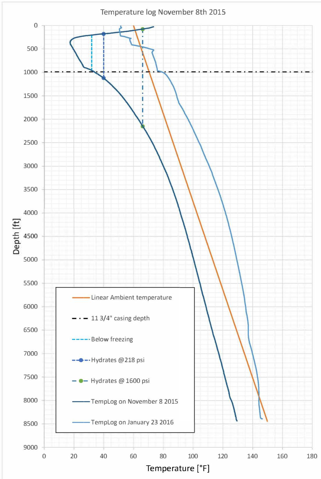
Figure 2.6: Temperature log from November 8<sup>th</sup> and January 23<sup>rd</sup> 2016
