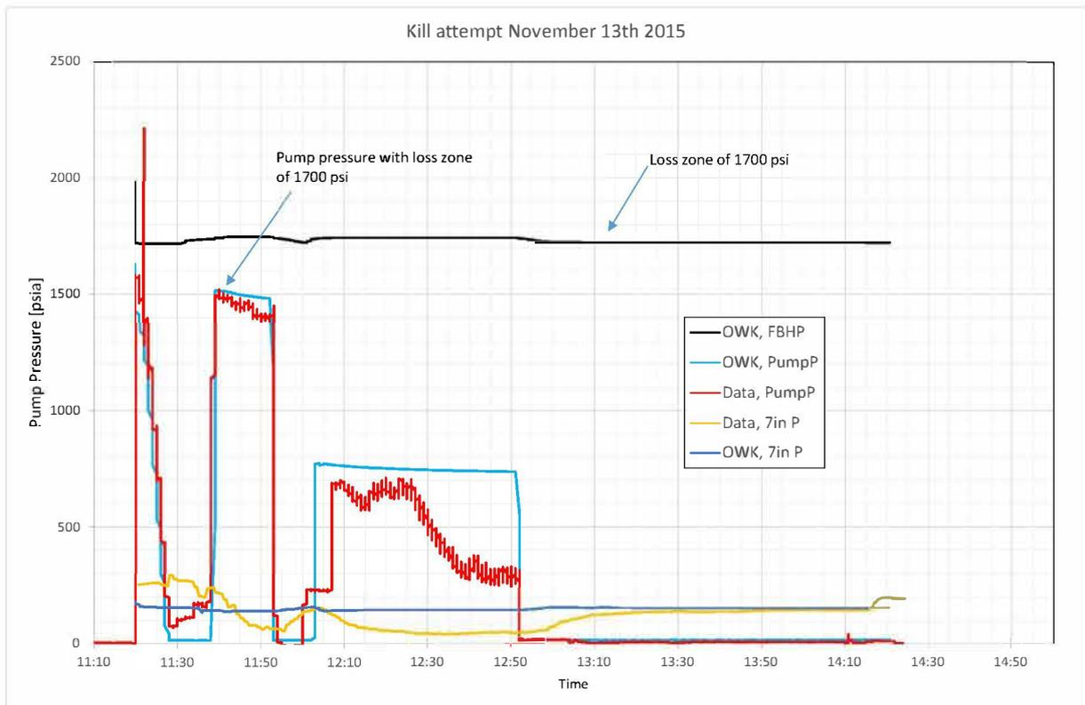
Figure 6.5: Pressures during pumping operation November 13<sup>th</sup> 2015, with losses
