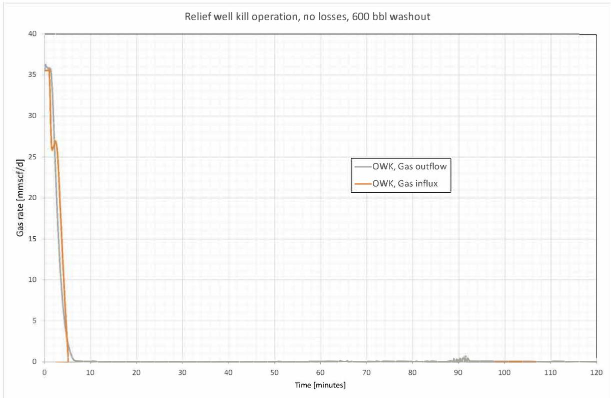
Figure B.7: Flow rates, RW kill, no losses, bottom washed out to 600 bbls
