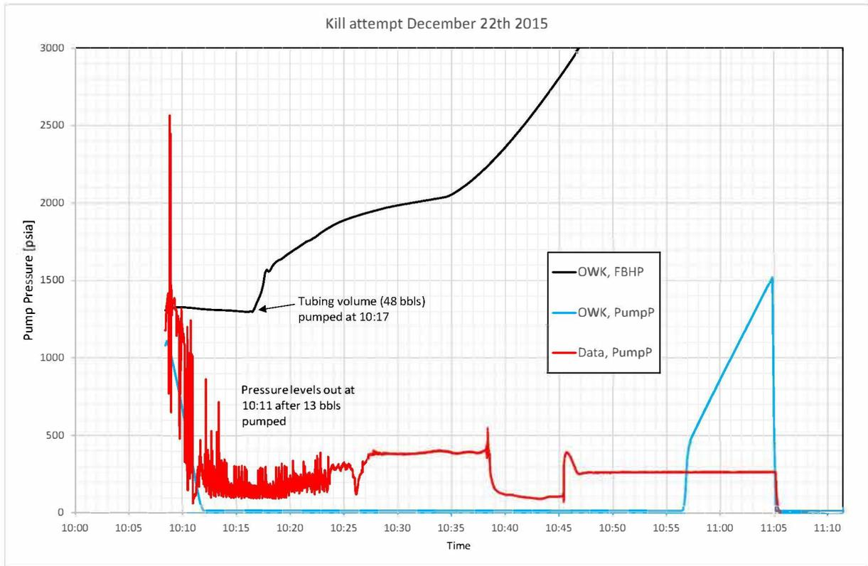
Figure 6.19: Pump rates during pumping operation December 22<sup>nd</sup> 2015
