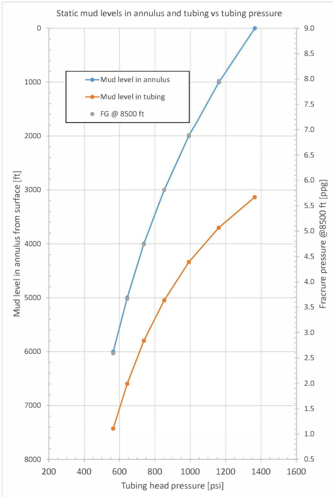
Figure 7.7: Liquid levels in SS25 after static kill using 9.0 ppg mud
