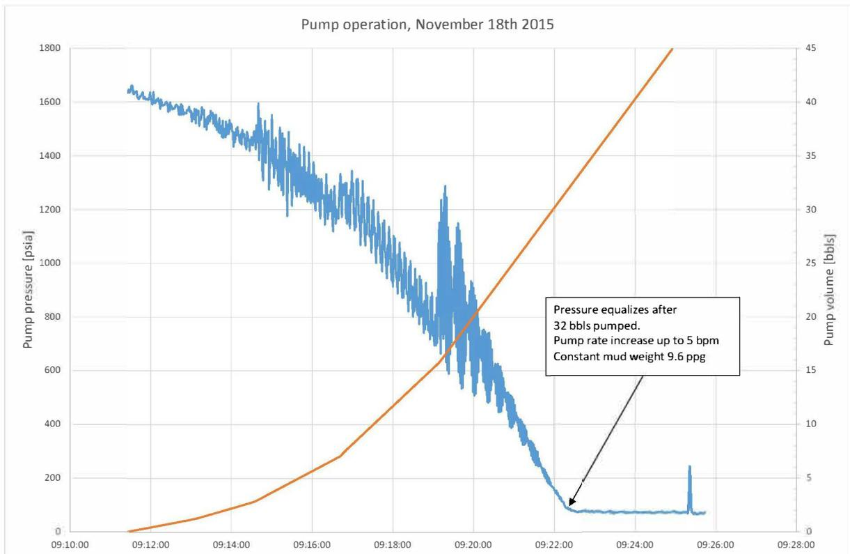
Figure 6.11: Pressure step-down during pumping operation November 18<sup>th</sup> 2015
