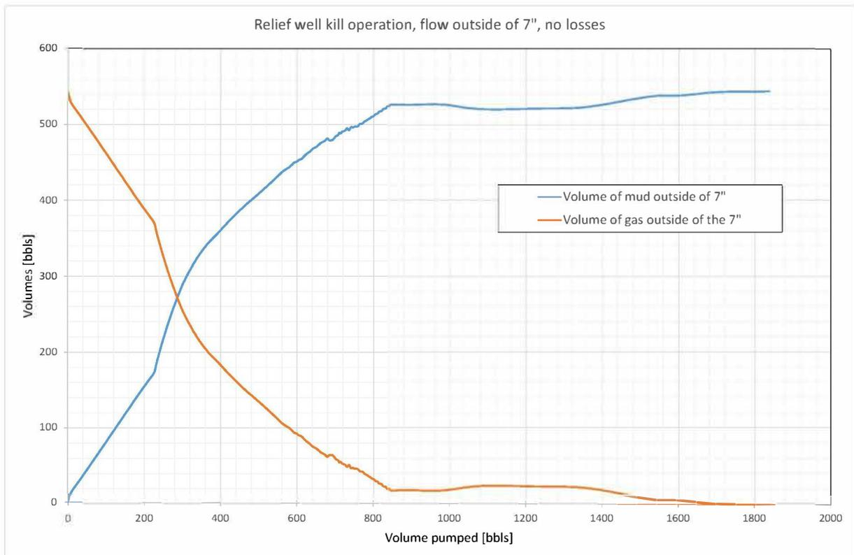
Figure 7.18: Fluid volumes during RW kill assuming flow outside the 7" csg
