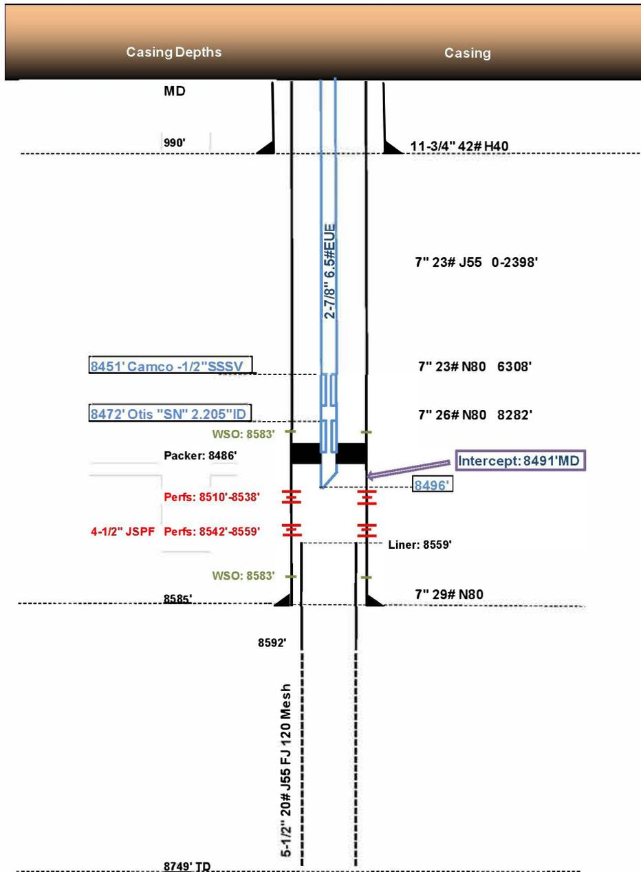
Figure 1.7: Wellbore schematic prior to perforation
