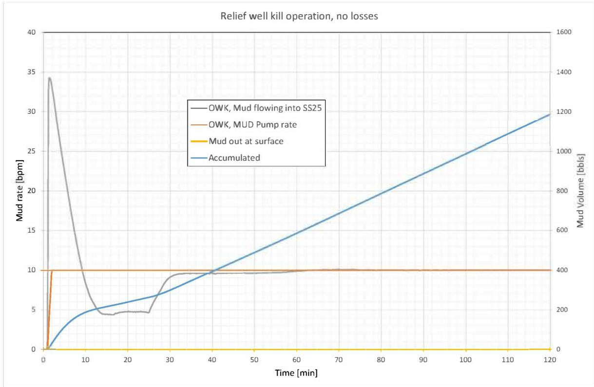
Figure B.9: Mud flow rates, RW kill, no losses, fracture gradient of 8 ppg
