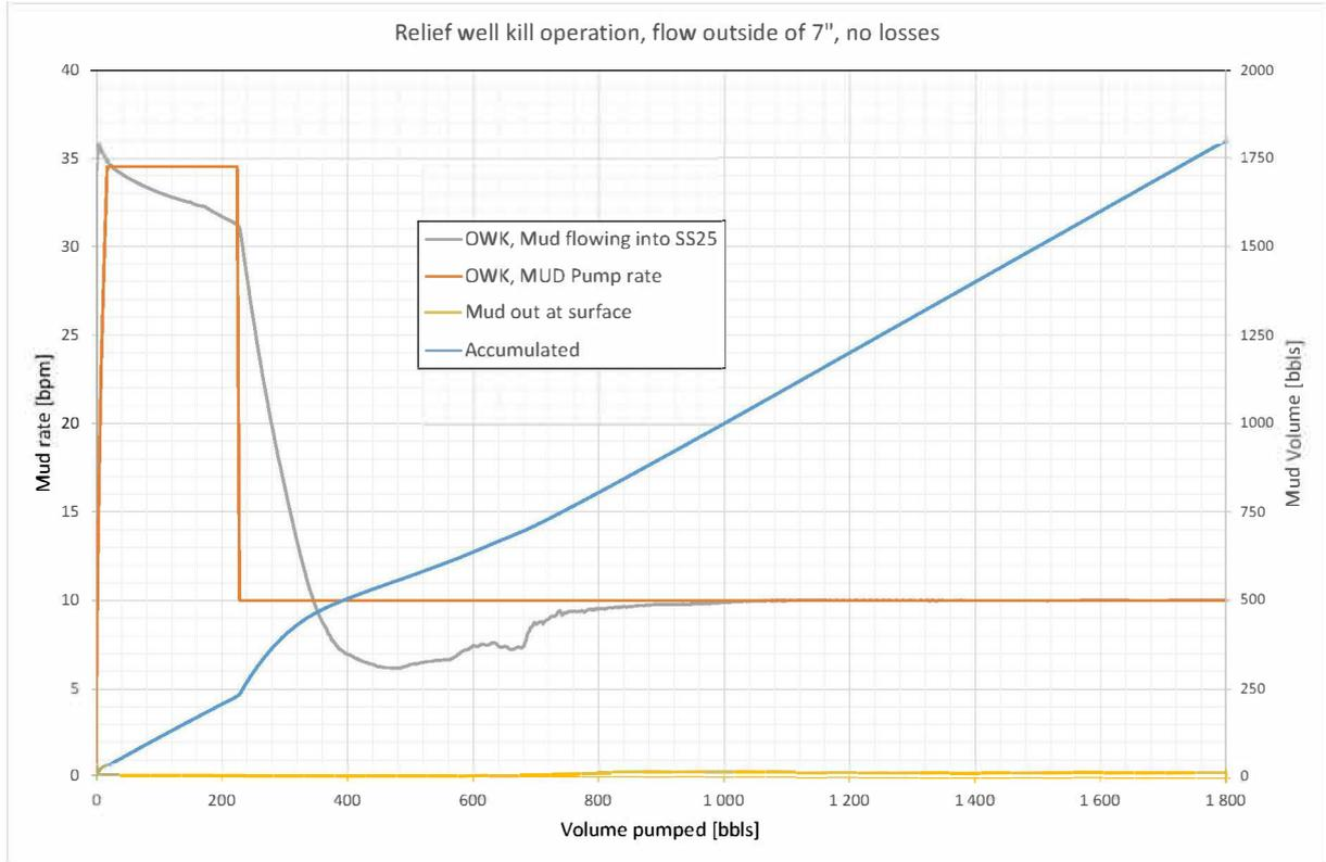
Figure 7.17: Mud rates and volumes during RW kill assuming flow outside the 7" csg
