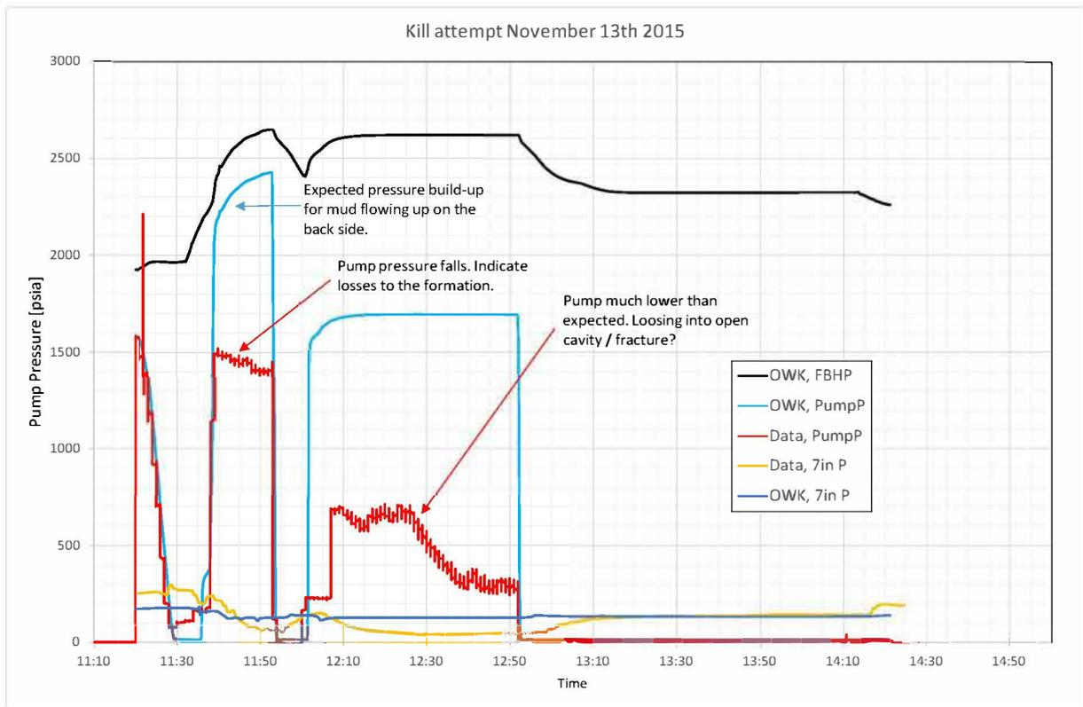
Figure 6.3: Pressures during pumping operation November 13<sup>th</sup> 2015
