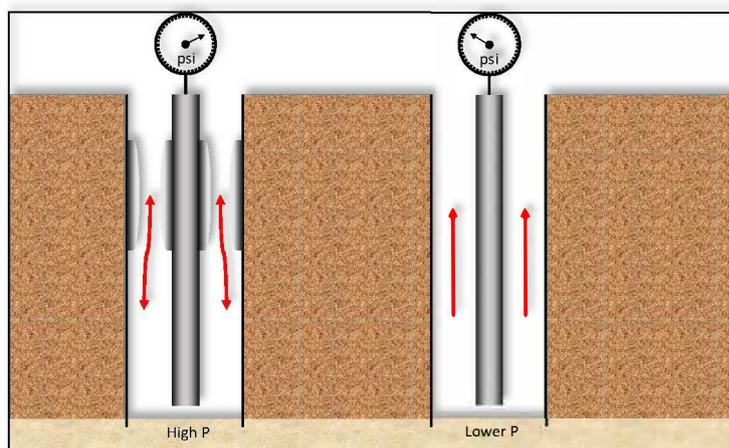
Figure 6.17: Effect of restriction on pressure reading
