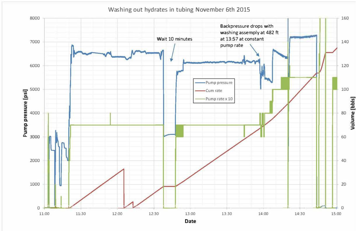
Figure 5.2: Rate and pump pressure during washing operation on October 6<sup>th</sup> 2015
