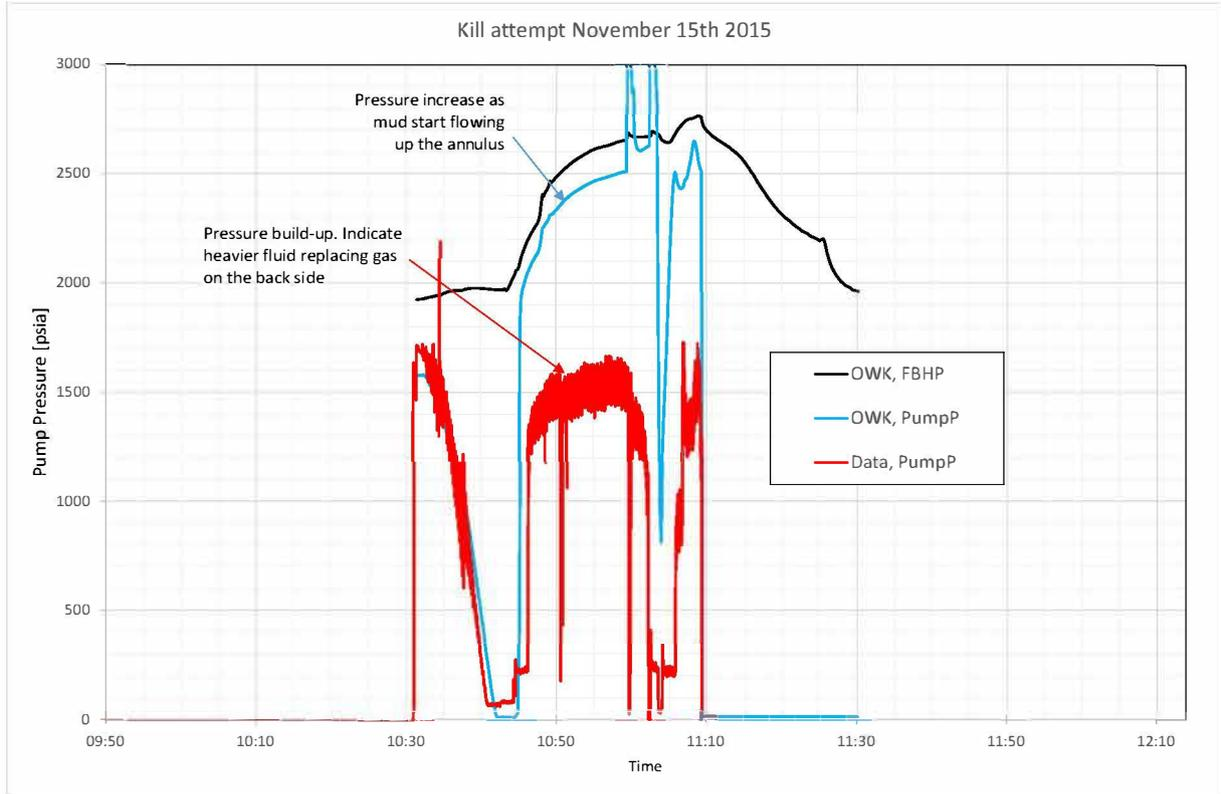
Figure 6.7: Pressures during pumping operation November 15<sup>th</sup> 2015
