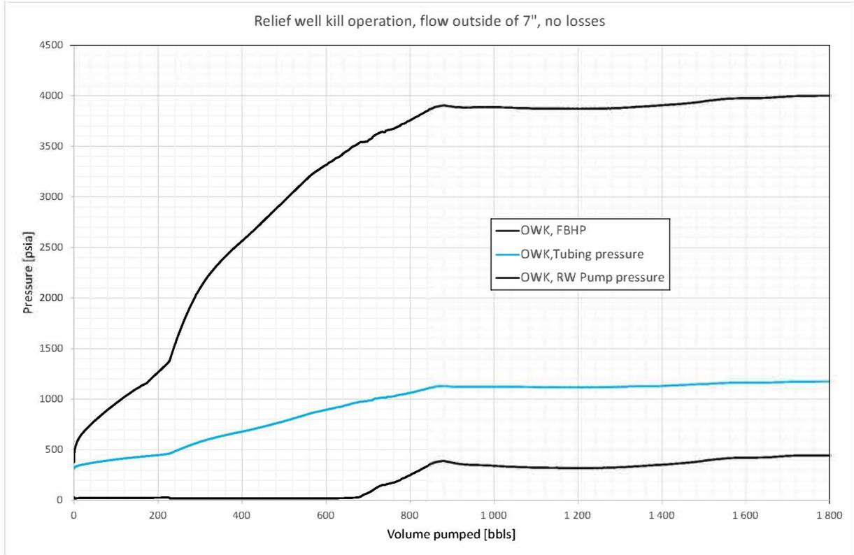
Figure 7.15: Pressures during RW kill assuming flow outside the 7" csg
