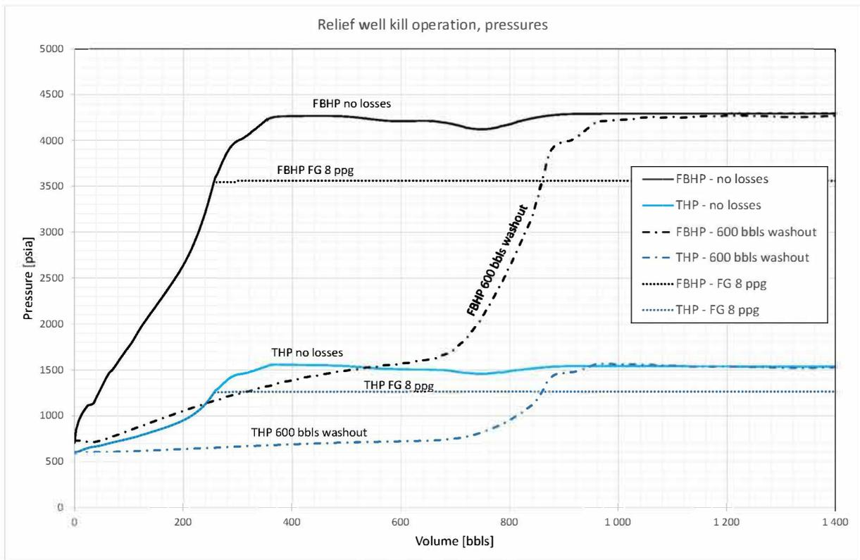
Figure 7.11: Relief well kill scenarios, FBHP and tubing pressures
