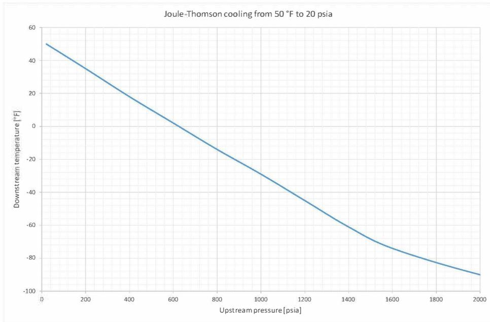
Figure 3.5: Joule-Thomson cooling from high pressure and 50 °F to 20 psia
