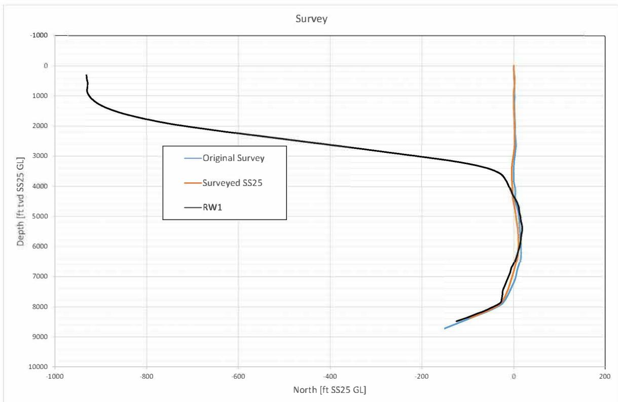
Figure 7.3: Relief well trajectory, North – TVD
