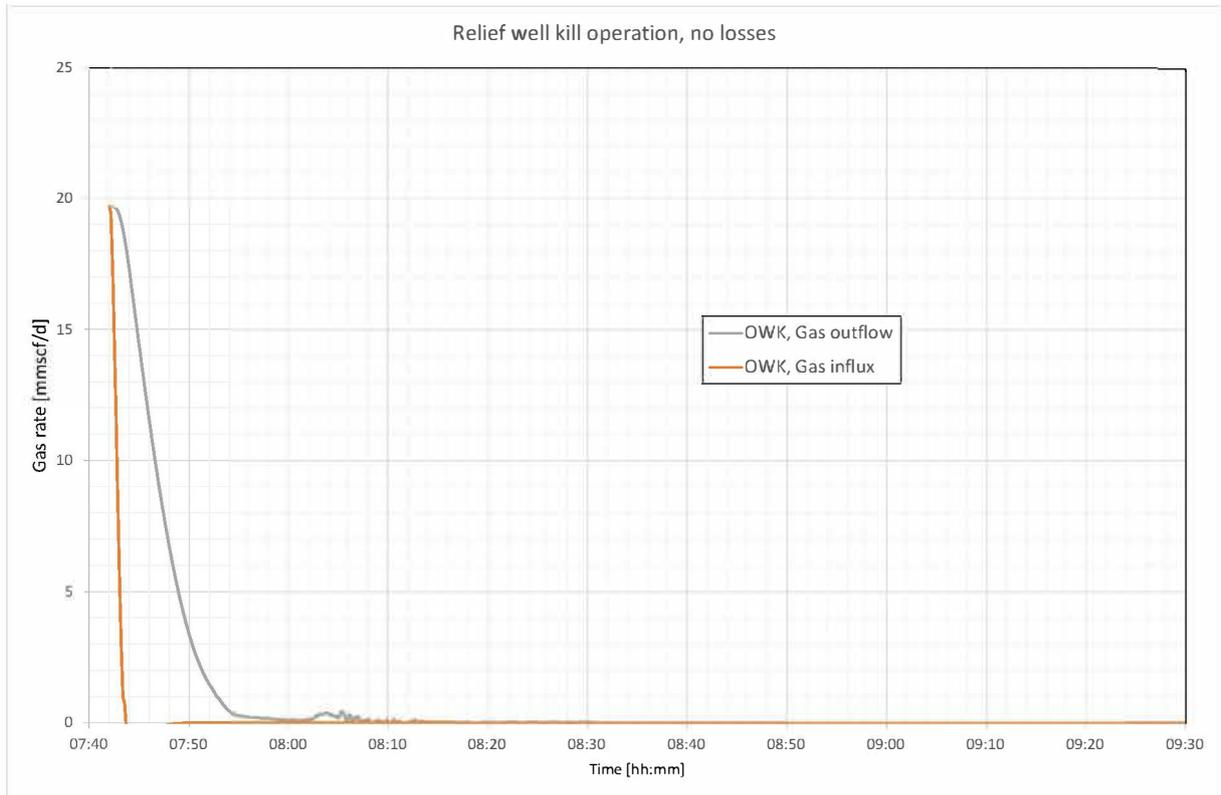
Figure 8.4: Relief well kill operation – gas flow rates
