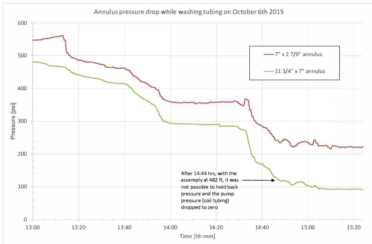
Figure 5.1: Pressure decline in annuli during washing operation on October 6<sup>th</sup> 2015
