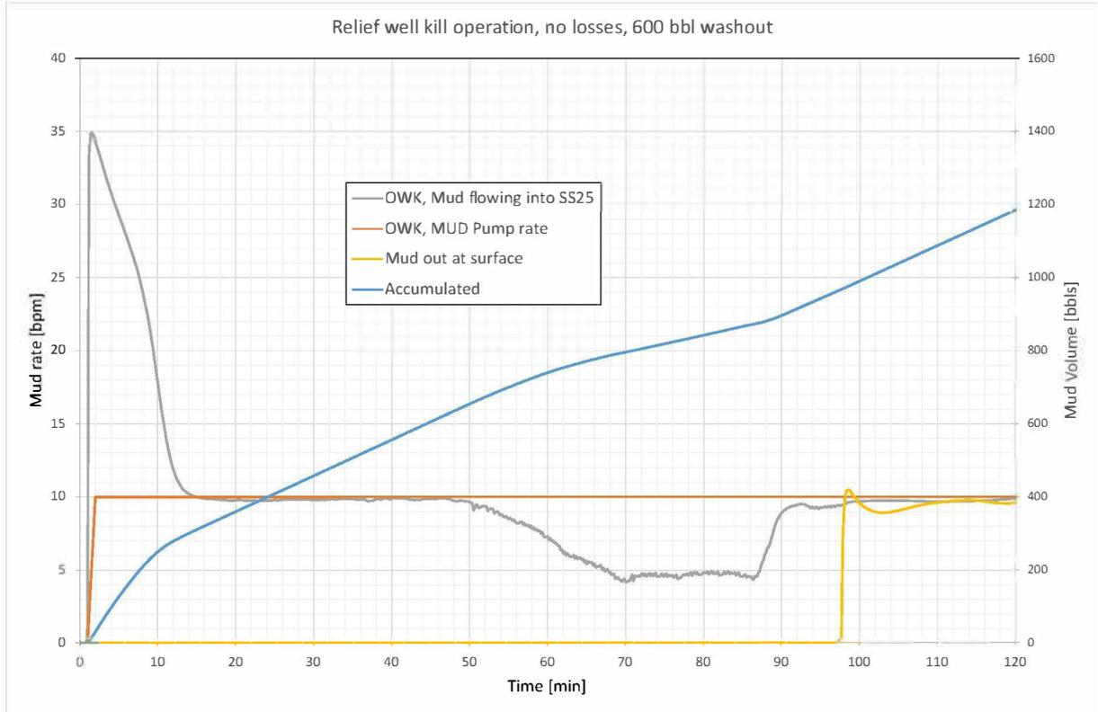
Figure B.5: Mud flow rates, RW kill, no losses, bottom washed out to 600 bbls
