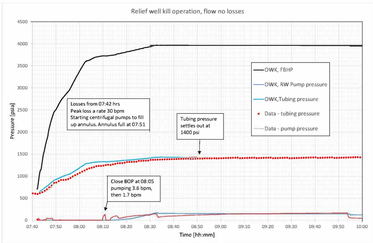
Figure 8.3: Relief well kill operation – pressures
