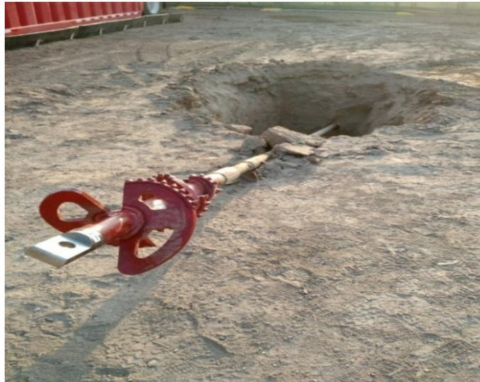
*Figure 13: Horizontal Directional Drill (HDD) Equipment*
