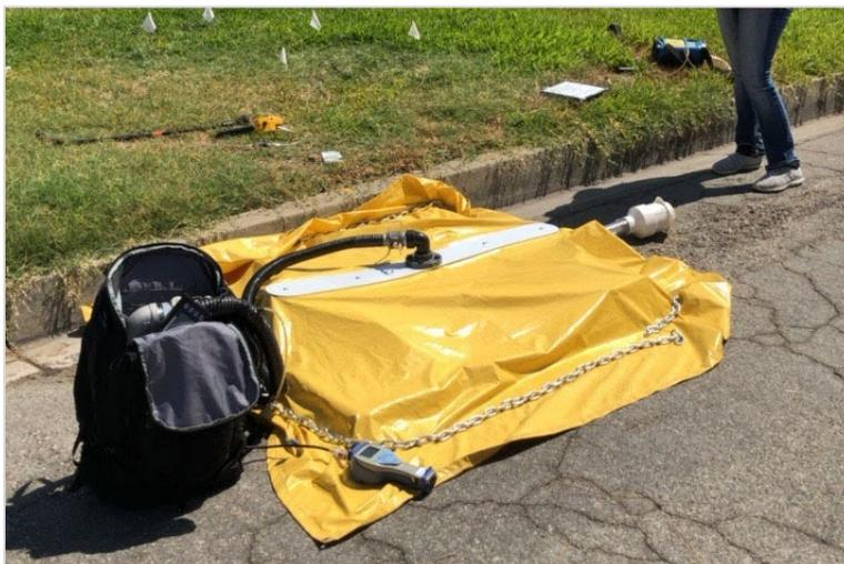
Using the "enclosure/chamber method. The high-flow device is housed in the backpack.
