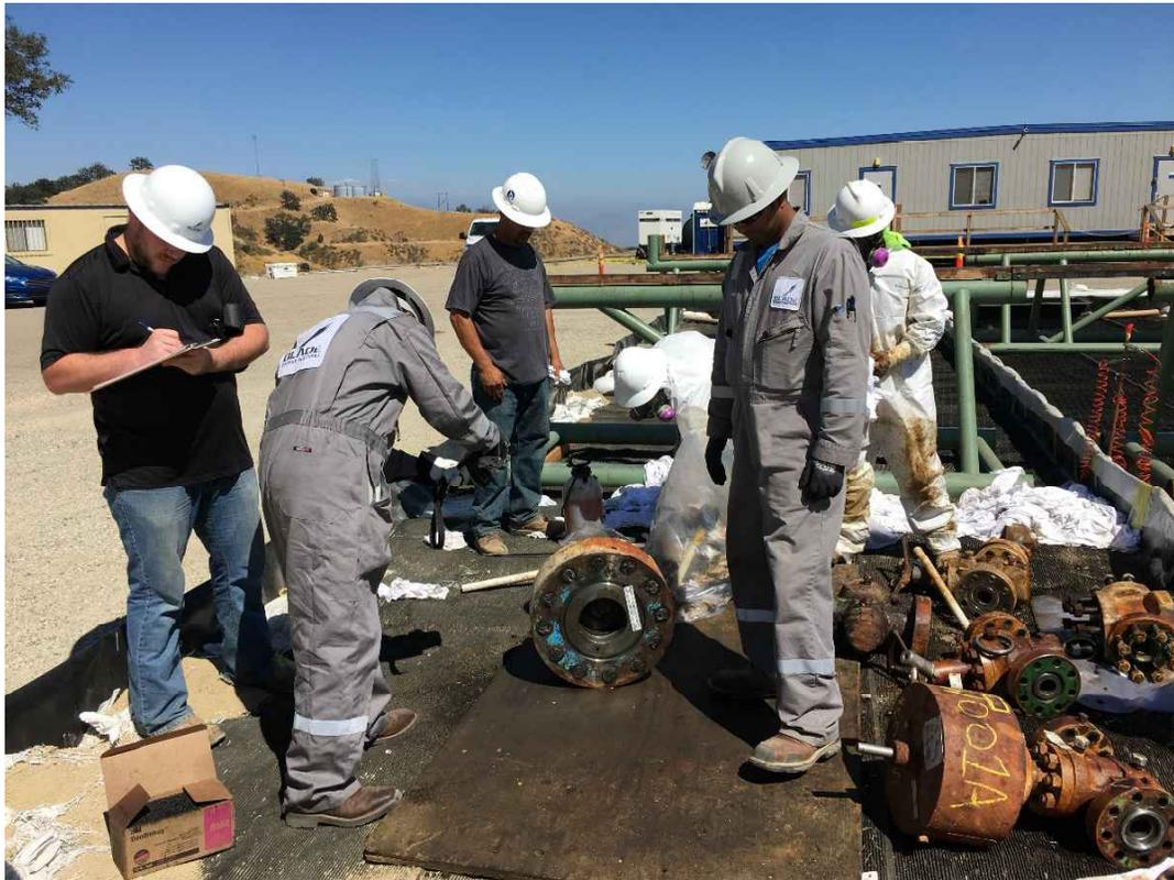
Figure 17: Tree Disassembly, Cleaning, and Inspection at PS-20
