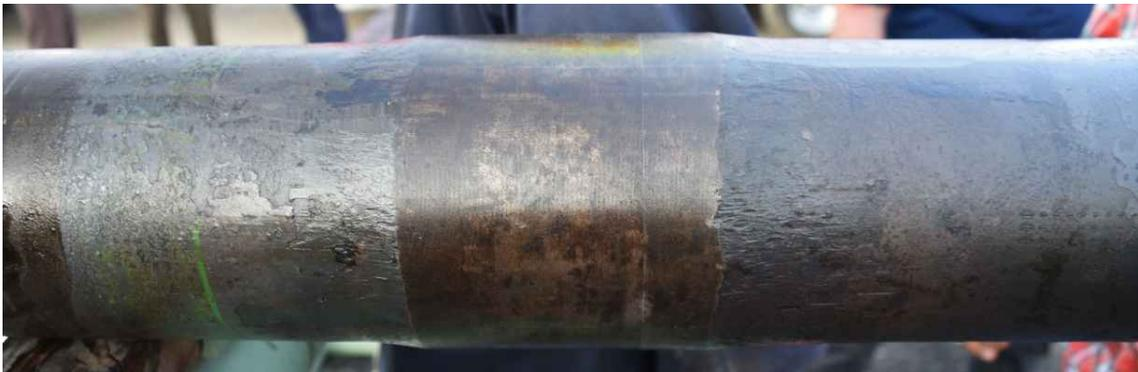
**Figure 32: Photo-Documenting the 7 in. Speedtite Connection (Box—Left, Pin-Right)**
