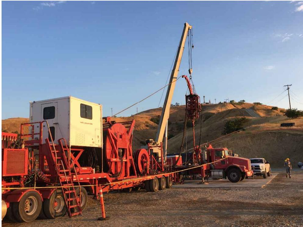
**Figure 15: Coiled Tubing Unit Rigged Up on SS-25**
