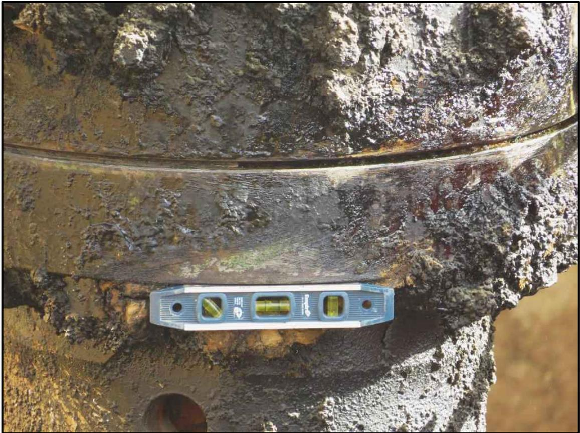
Figure 40: Level Affixed to Bottom of Bradenhead for Visual Confirmation of Surveyed Plumbness
