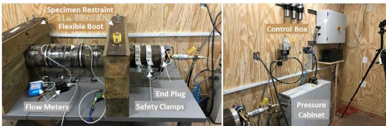
**Figure 22: Connecting Test Setup**
