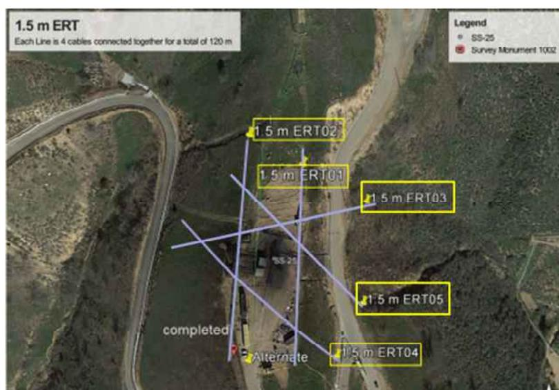
**Figure 2: Survey Line Orientation Example—1.5 m Spacing Electric Resistance Tomography Survey**
