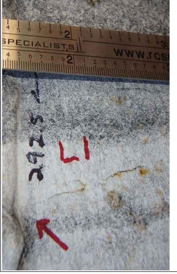
Description : Surface lamination detected at 292.5 degrees below girth weld
