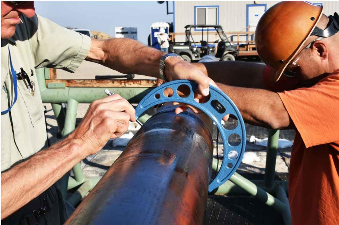
**Figure 31: Examining and Dimensioning 7 in. Speedtite Connection**
