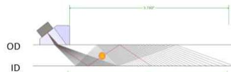
How the same reflector is represented in Phased Array views.
