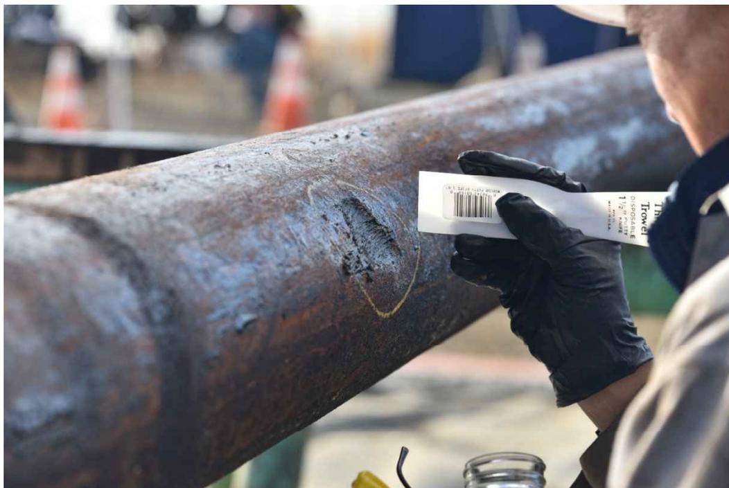
Figure 26: Inspecting and Collecting Scale Sample from a Joint of 7 in. Casing at SS-25
