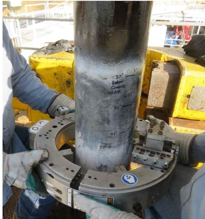
Figure 23: Cutting the 7 in. Casing
