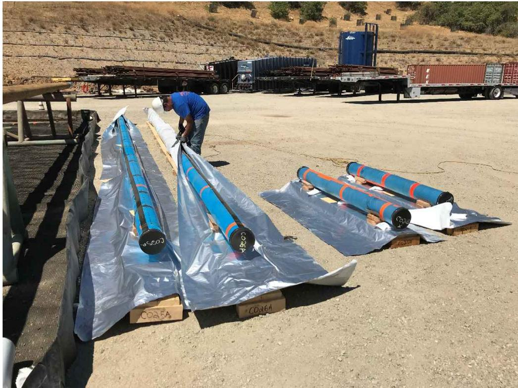
Figure 35: Preparing to Crate Two Full-Length Joints of 7 in. Casing and Two Connections at PS-20
