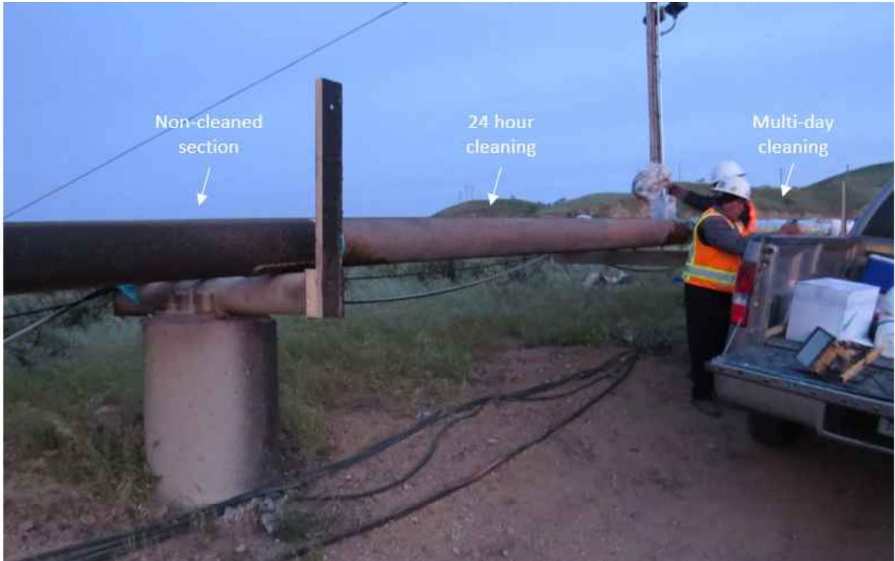
**Figure 40: Flow Line for SmartStripPRO™ Evaluation**
