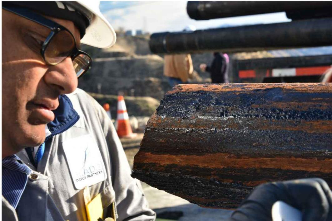
Figure 27: Inspection of a Joint of 7 in. Casing at SS-25
