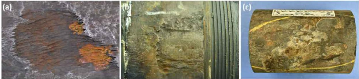
Figure 10: Corrosion Features from (a) C021, (b) C024B, and (c) C025
