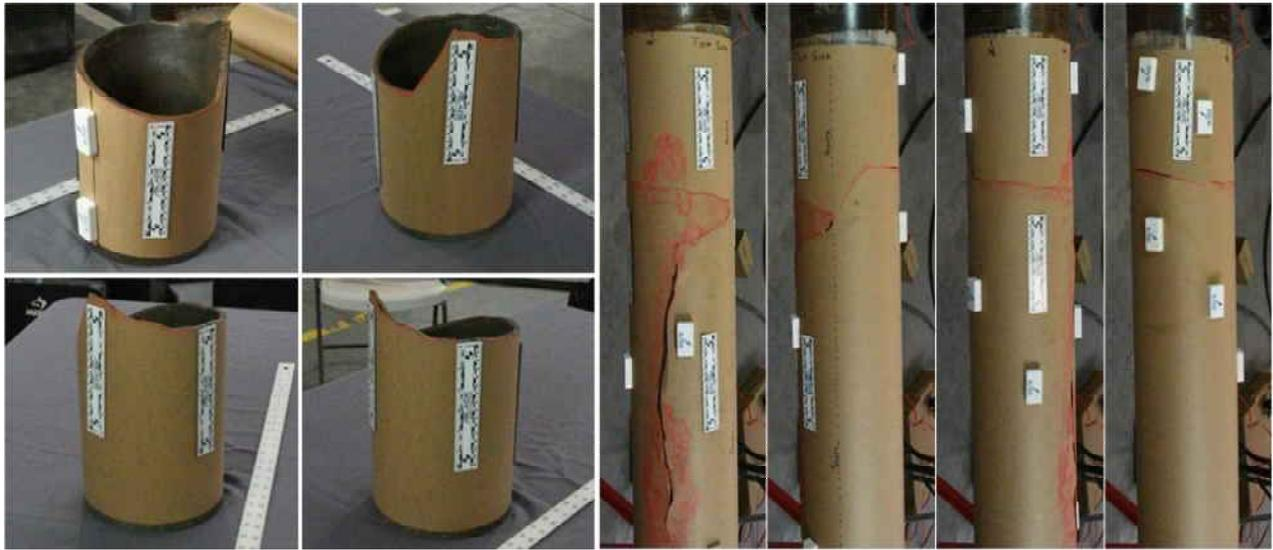
Figure 12: Completed Paper Reconstruction of C022B and C023A1
