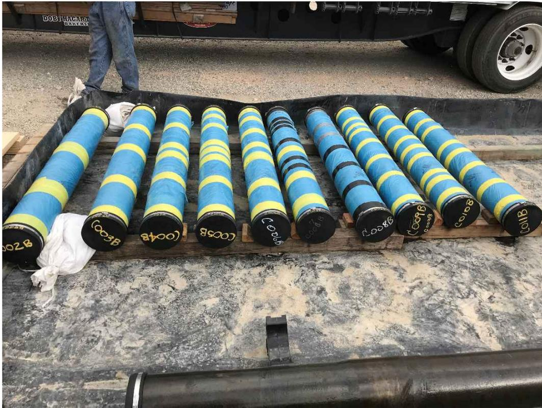
Figure 33: 7 in. Connection Sections Wrapped in Volatile Corrosion Inhibitor at PS-20
