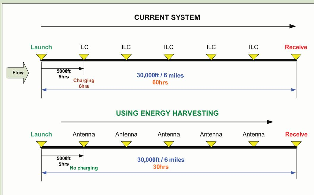
*In 2019, the project team demonstrated an onboard energy harvesting module that enabled an Explorer model in-line inspection robot to avoid the need for in-line charging and dramatically reduce inspection times.*
